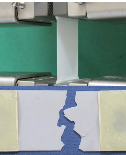
Determination of the strength of 90 µm thick 3YSZ substrate in a tensile test.
