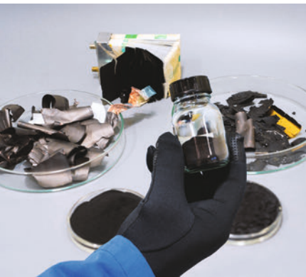
Black mass of end-of-life batteries to be processed for the recovery of valuable metals.
