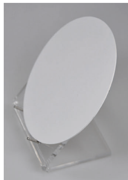
Disk-shaped solid state electrolyte made of sodium-beta alumina.
