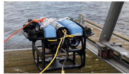
Underwater robot for photo documentation (source: Fraunhofer IGD).
