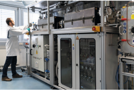
Roll-to-roll CVD coating system for continuous fiber coating.
