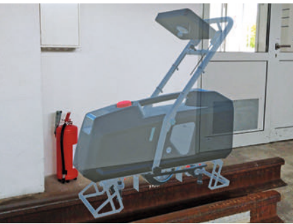
Virtual CAD model of the SoniQ Rail Explorer in the data glasses.
