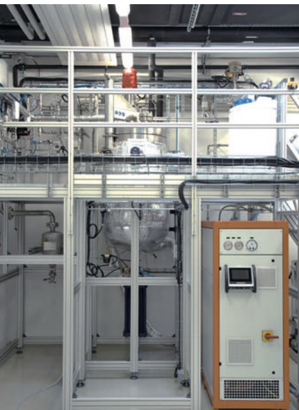
Pilot plant for Li recovery using the COOL process.
