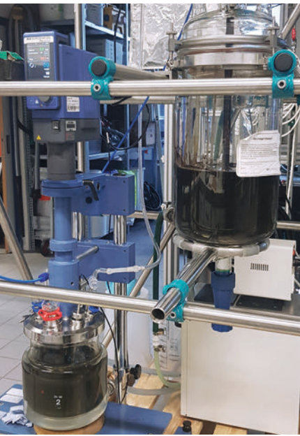
Test system for circulation stripping.
