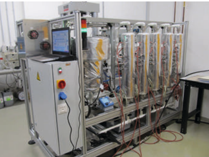
Gas separation system, for external use.
