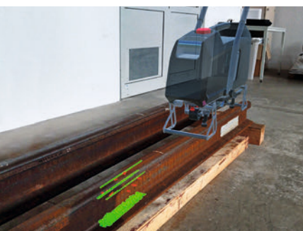
Representation of mesh data and the overlay with the real test object.
