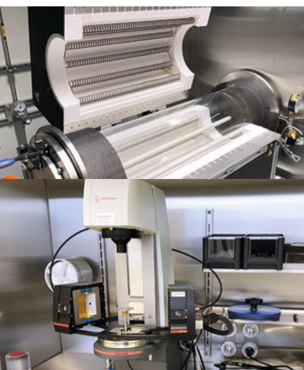
Measuring samples sensitive to moisture and air. Top: Furnace integrated in Ar-Glovebox. Bottom: Rheometer integrated in Ar-Glovebox.
