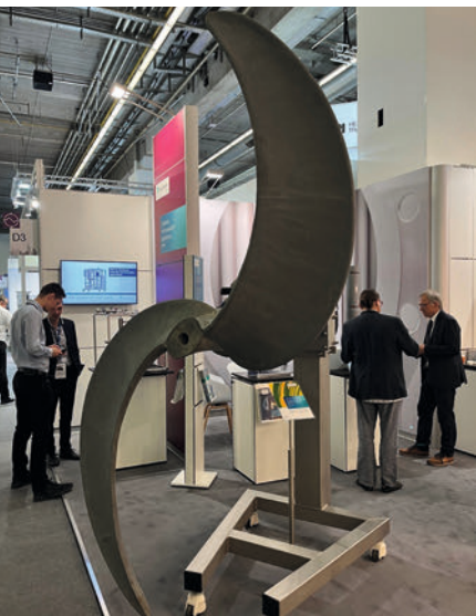
Pilot impeller on a trade fair stand after the two-year application test.
