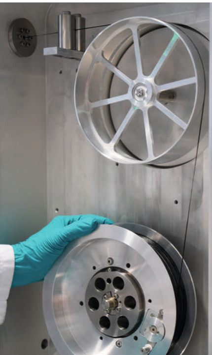
Winding unit with processed endless fiber roving.
