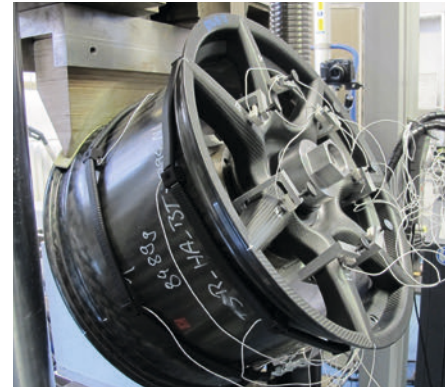
CfK rim testing with acoustic emission analysis.
